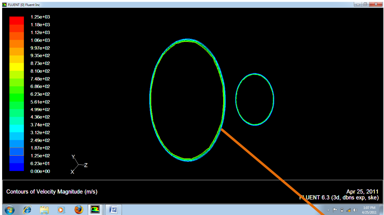
Figure 3.7: Inlet velocity contours for low bypass turbofan engine.
