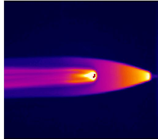
Influence of roughness on laminar to turbulent transition
