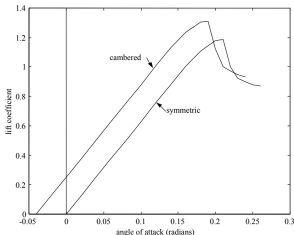
Figure 1.1: Typical lift curves for symmetric and cambered airfoils.
