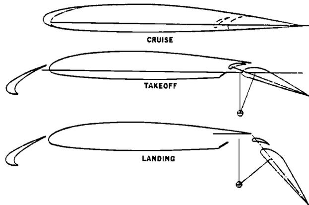
Figure 1.2: Typical double-slotted flaps/leading-edge slat high-lift system (from *Shevell*, 1979).
