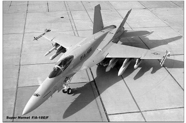
Fig. 16 Typical high-performance military aircraft with external stores.
