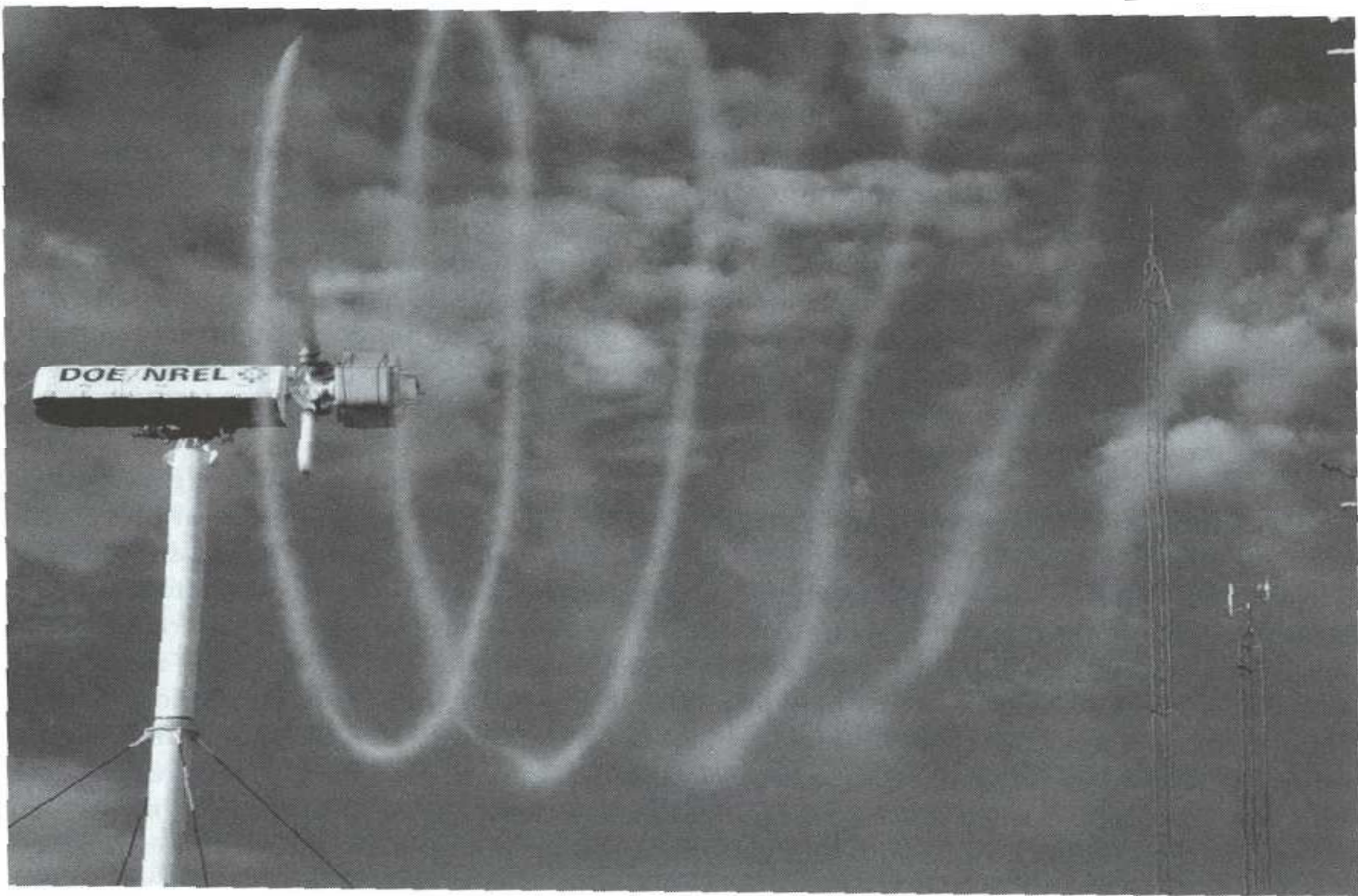
Figure 13.20 Photograph of the vortical wake behind a horizontal axis wind turbine rendered visible using smoke injection. Notice the skewed wake resulting from the wind gradient and the effects of the tower shadow. Source: Photo courtesy of NREL.
