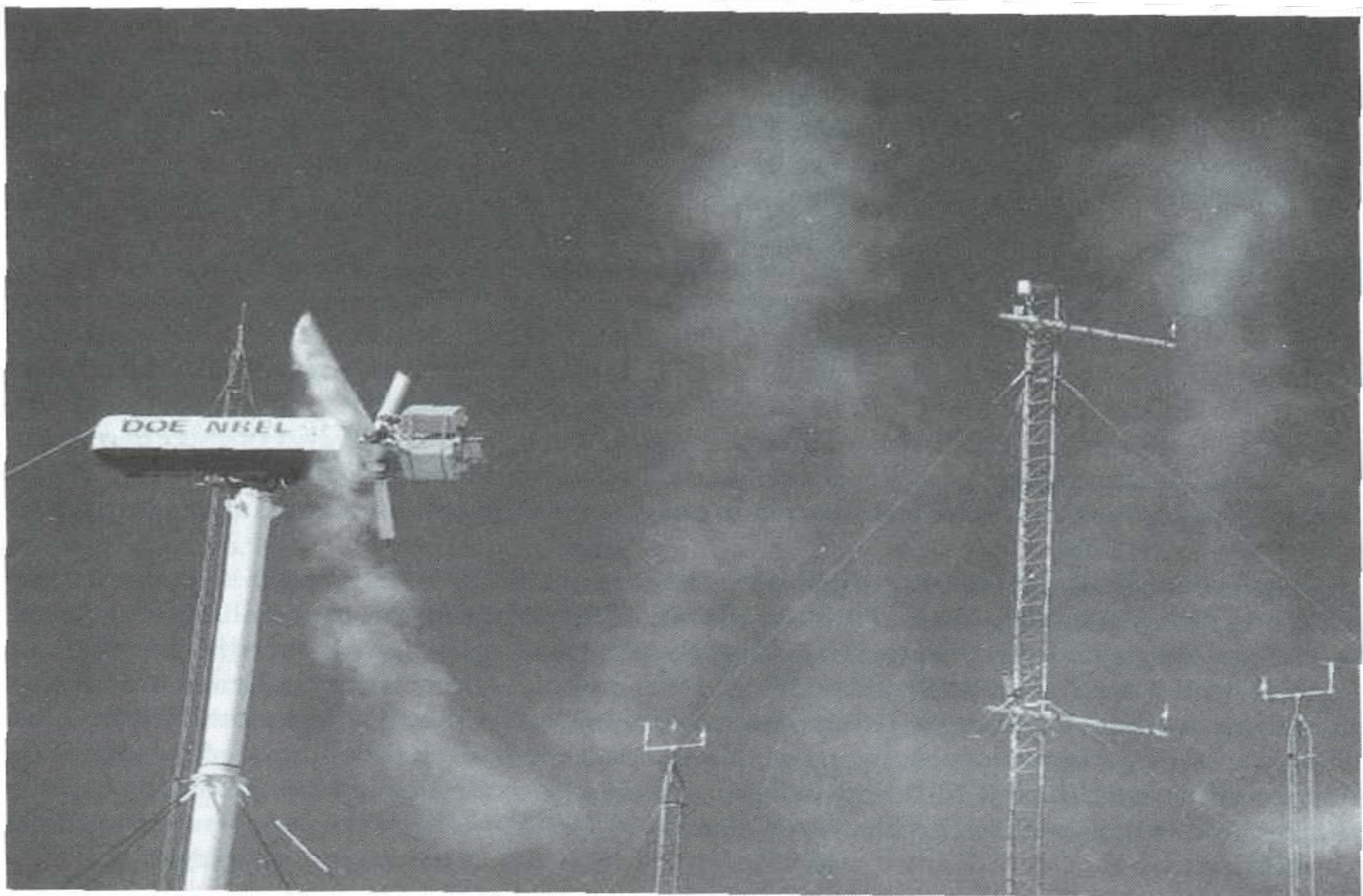
Figure 13.28 The onset of stall on the turbine produces highly nonlinear aerodynamic loads and a turbulent wake structure. Source: Photo courtesy of NREL.
