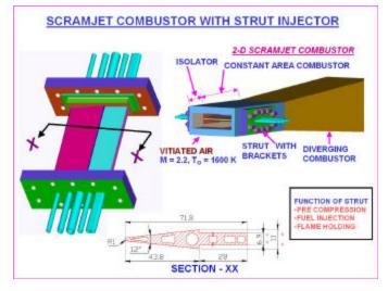
Fig 2: Strut injector
