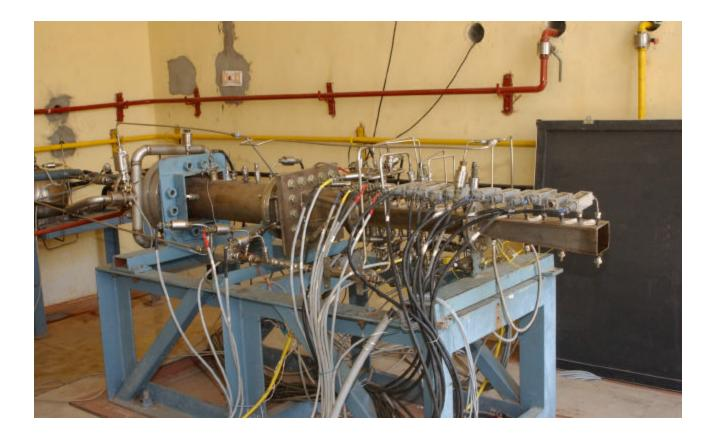
Fig 1: Scramjet Combustor Mounted on the test facility
