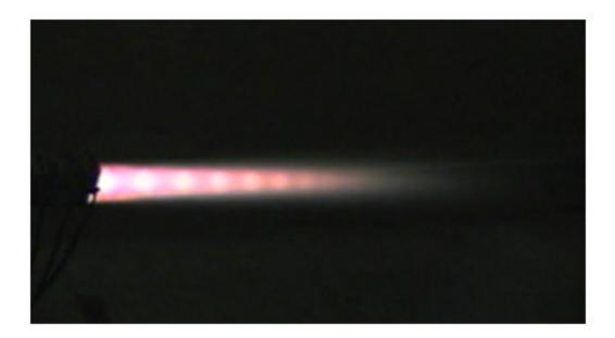
PLATE 1: Supersonic Flame during Pilot Hydrogen injection
