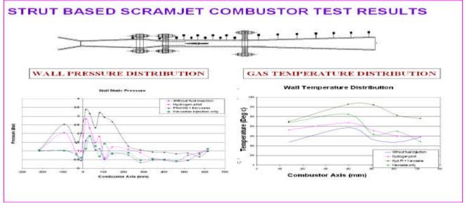
FIGURE 3: Pressure and Temperature Distribution
