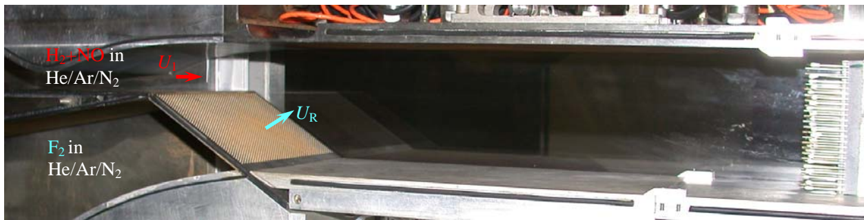
Fig. 1. The supersonic shear-layer facility expansion-ramp flow geometry
