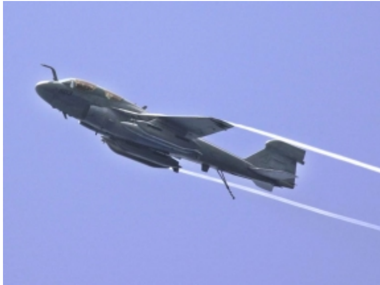
Figure 1.4: Tip vortices trailed behind an E/A-6B Prowler [40]
