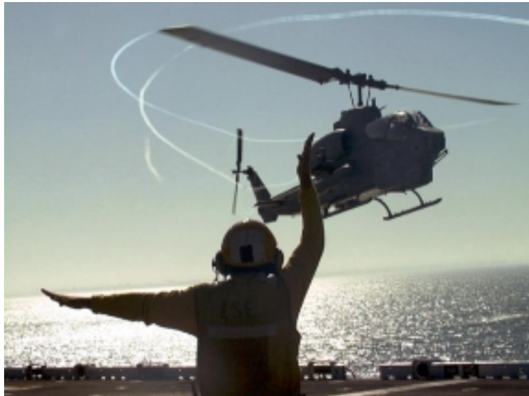
Figure 1.5: Tip vortices trailed behind the blades of an AH-1W Super Cobra [40]
