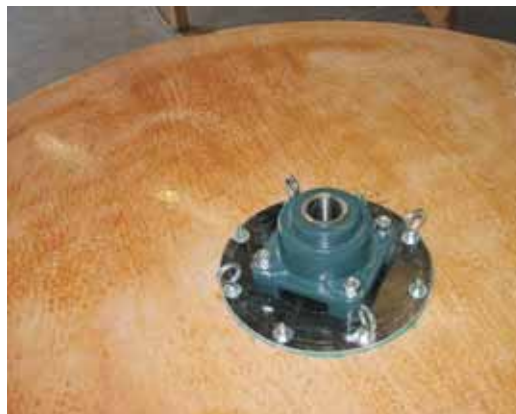
The middle bulkhead with main bearing attached. The eyebolts had cables connected to the lower bulkhead rim to carry the cylinder weight.
