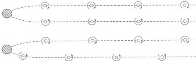
Figure B. Double rows of alternating vortices; symmetric (upper) and asymmetric (lower) arrangements. (Reproduced from Theodore von Kármán, Aerodynamics: Selected topics in the light of their historical development , Cornell University Press, 1954.)
