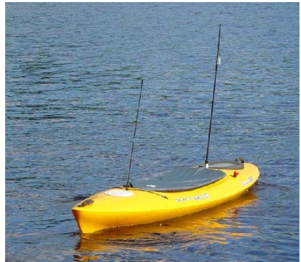
Fig. 6: Autonomous kayak test platform
