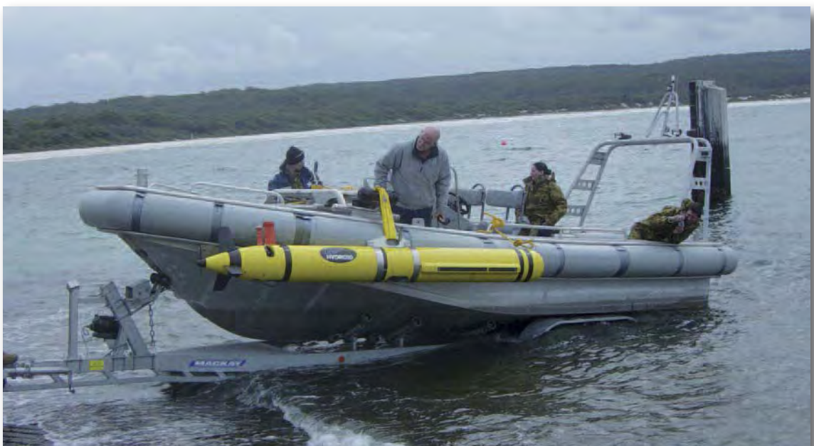
REMUS 600 provides a detailed maritime survey and mine detection and classification capability in the 30m to 200m depth range, although the vehicle can operate down to 600m. It is fitted with a range of sensors and runs on re-chargeable batteries
