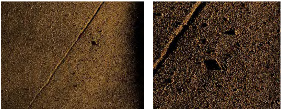
Left: A section of HISAS 1030 on port swath with exercise object (2 m long, 53 cm diameter cylinder) Water depth 10-13 meters, HUGIN 1000 depth 3 meters, range 15-95 meters. Right: 10x10 meter detail around the exercise object
