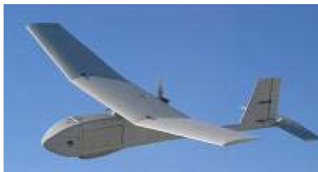
Figure 1. RQ-11 Pathfinder Raven UAV (From OSD, 2009)
